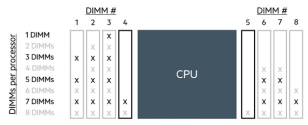
**NOTE:** Chart to be read from left to right. For example, when installing four (4) DIMMs on a processor, DIMMs 2, 3, 6, and 7 should be populated.
