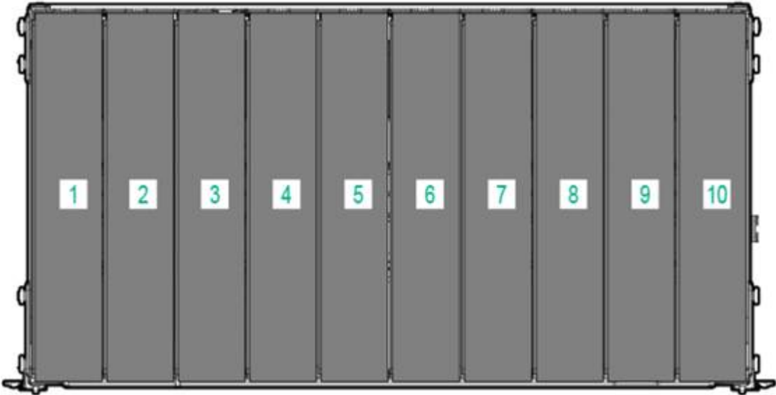
Server tray bay numbering (1-10) - Front View Populate trays from right (Bay 10)-> left (Bay 1)
